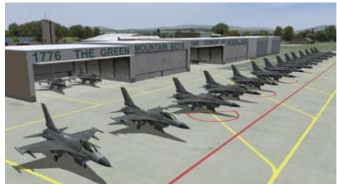
To geolocate many of the elements on the airfield terrain to match the ones on the actual airfield, an interactive panoramic view was created from photos taken at the site as a reference, using photo-stitching software. This panoramic view was then mapped onto a 3D cylindrical model, resulting in a 360-degree virtual view, or model (shown below) that could be examined as a reference for placing models on the terrain.
