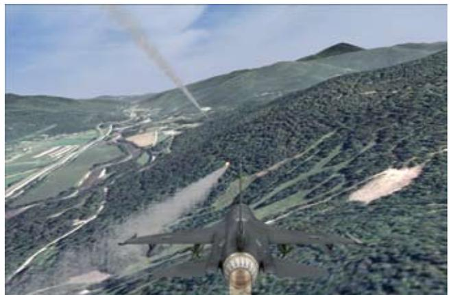
All site-specific models were created with textures derived from high-resolution photographs taken at the site at ground level with a 10-megapixel camera. The models were built with industry standard 3D modeling tools such as Autodesk Maya and 3ds Max. Content from MetaVR's 3D model libraries is also used on the terrain.
