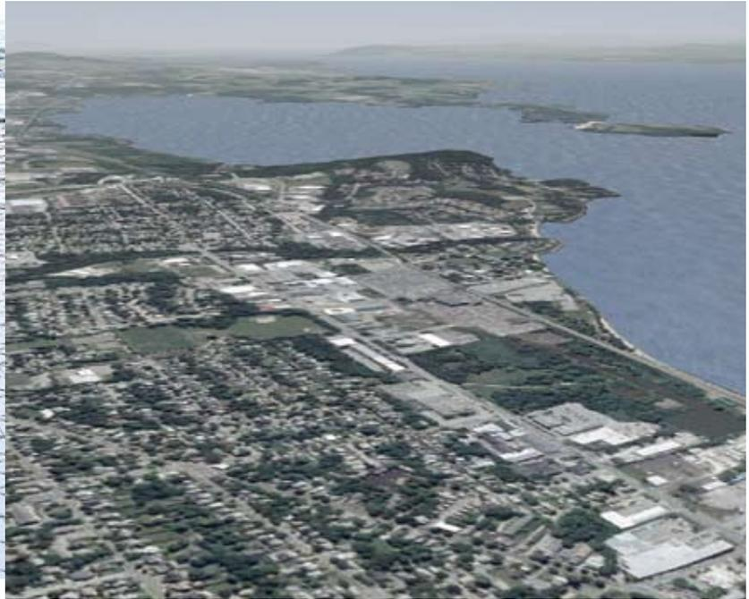
MetaVR Terrain Tools for ESRI ArcGIS was used to create the terrain mesh, which includes a high resolution representation of the Lake Champlain coastline. At runtime, VRSG Metadesic generates multi-textured, animated, normal-mapped water surfaces in the cutout regions identified as water. The terrain tiles seamlessly match with the water tiles generated by VRSG.
