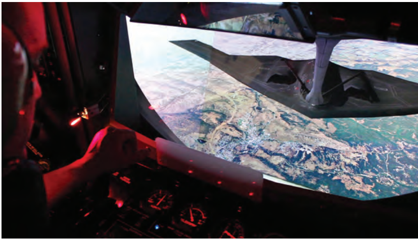
Inside the boom pod of the KC-135R Air National Guard (ANG) Boom Operator Simulator System (BOSS) with MetaVR visuals. Photo courtesy of FAAC, Inc.
